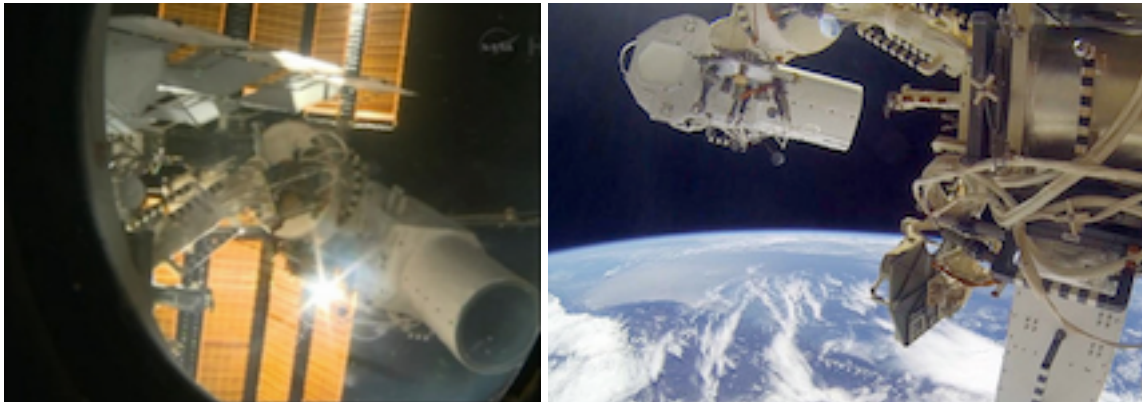
GoPro camera view of UrtheCast's high- (upper left) and medium-resolution (lower right) commercial video cameras mounted on the International Space Station
